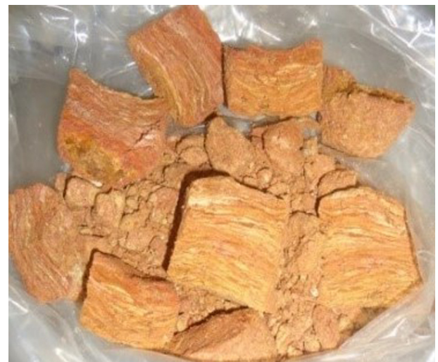
Fig. 3. San Diego IC residual soil sample photograph.
